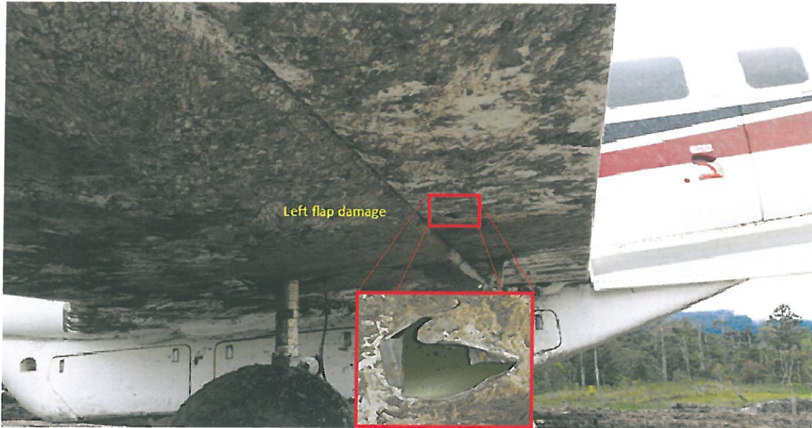
Figure 5: Puncture in the left flap skin
