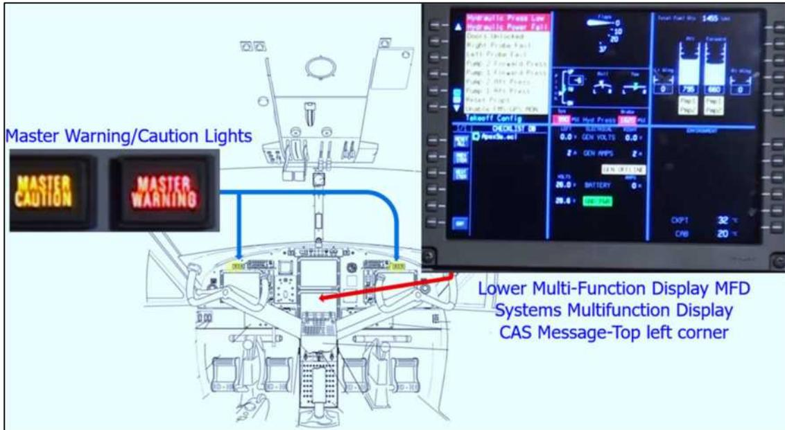
Figure 5: Crew alerting system display.
