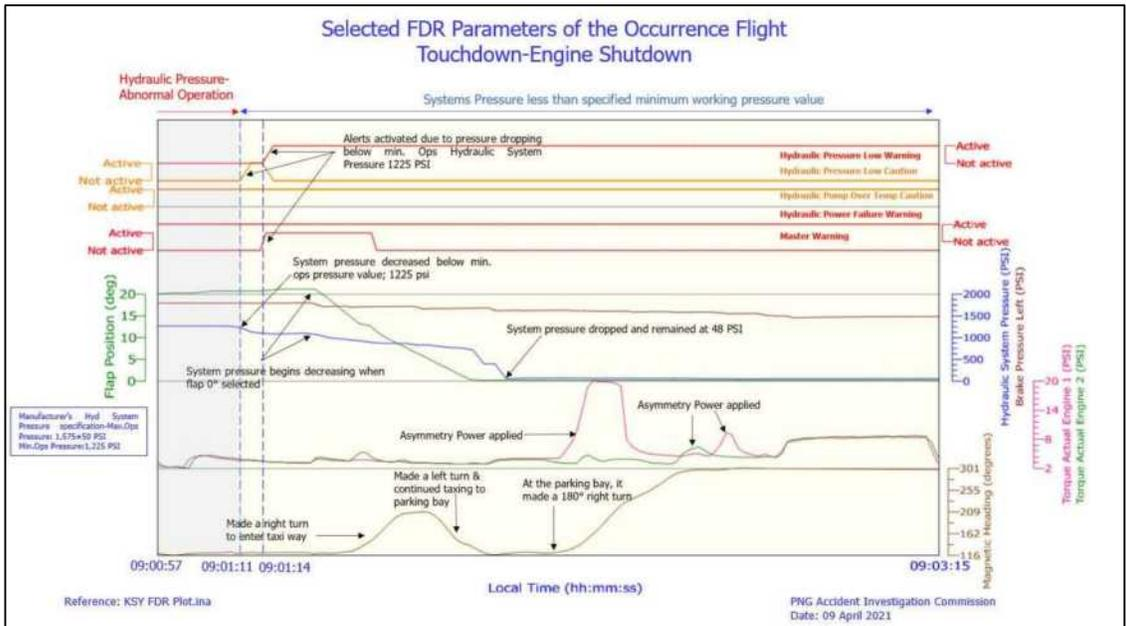
*Figure 9: FDR Recorded parameters of the occurrence flight from touchdown to complete stop.*
