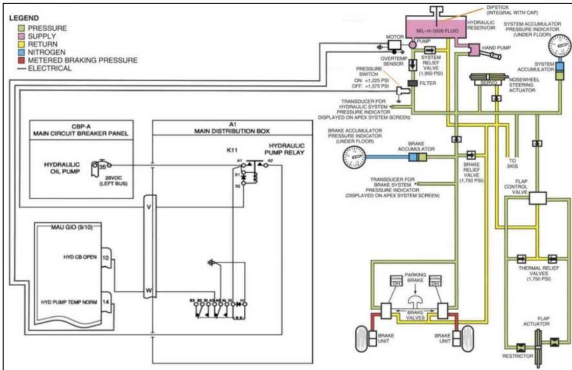
Figure 4: Hydraulic electro-mechanic system. (Refer Appendix A-1 and A-2 for original diagrams)
