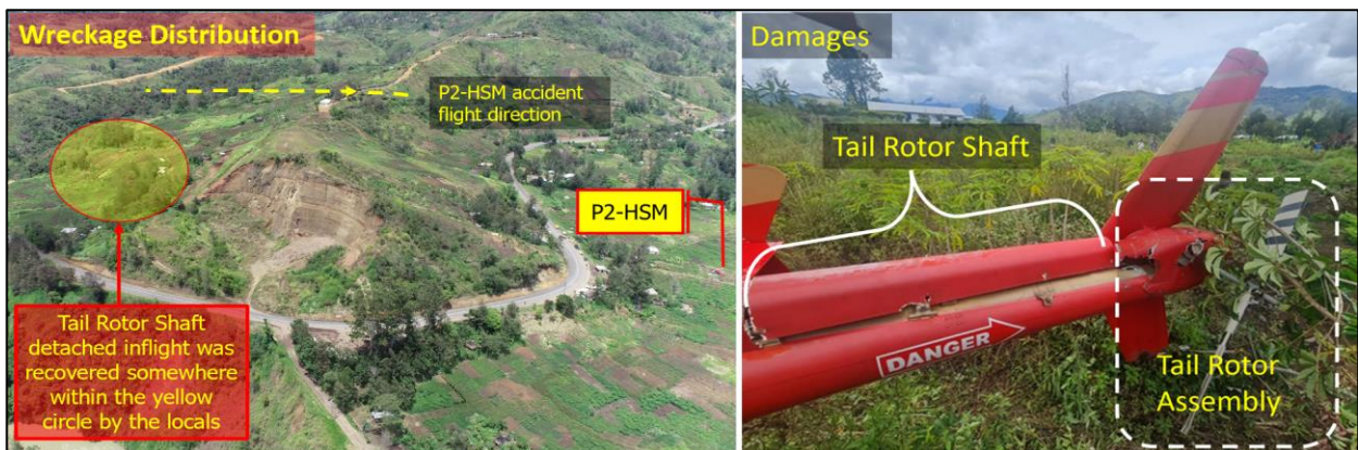
Figure 3: P2-HSM wreckage distribution and the damages sustained
