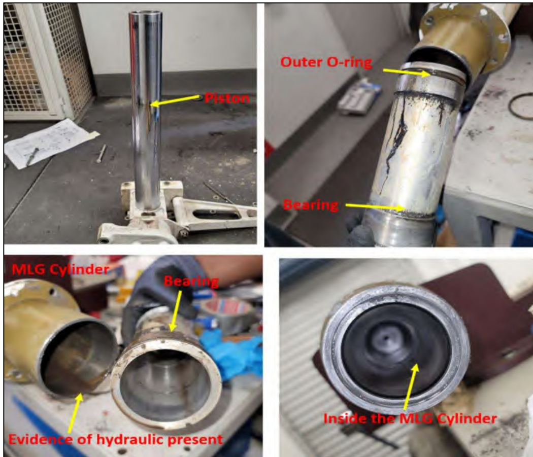
Figure 16. Observations on the MLG oleo strut.
