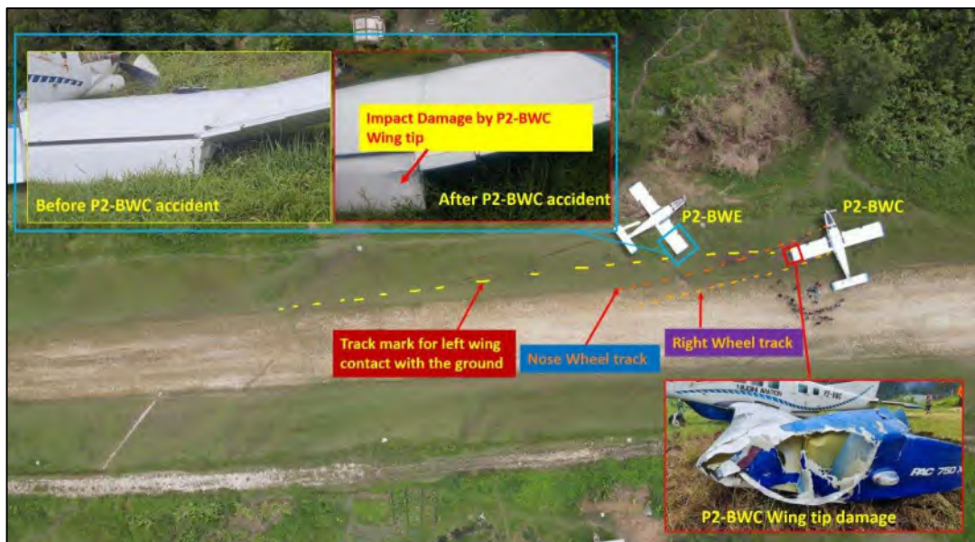
Figure 3. Damage caused to P2-BWE by P2-BWC.
