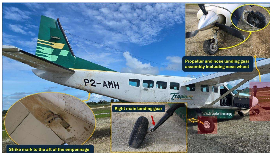
Figure 6. Observation of the damage to the aircraft.
