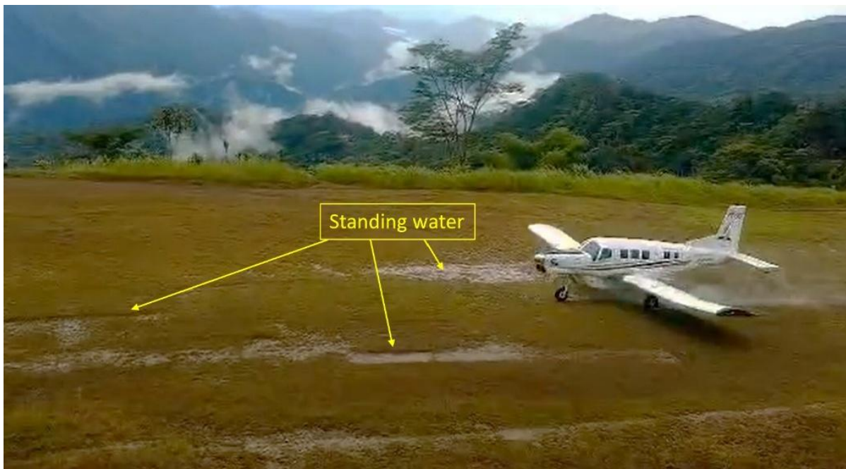
Figure 6. P2-SDA encounters standing water on Runway 02.
