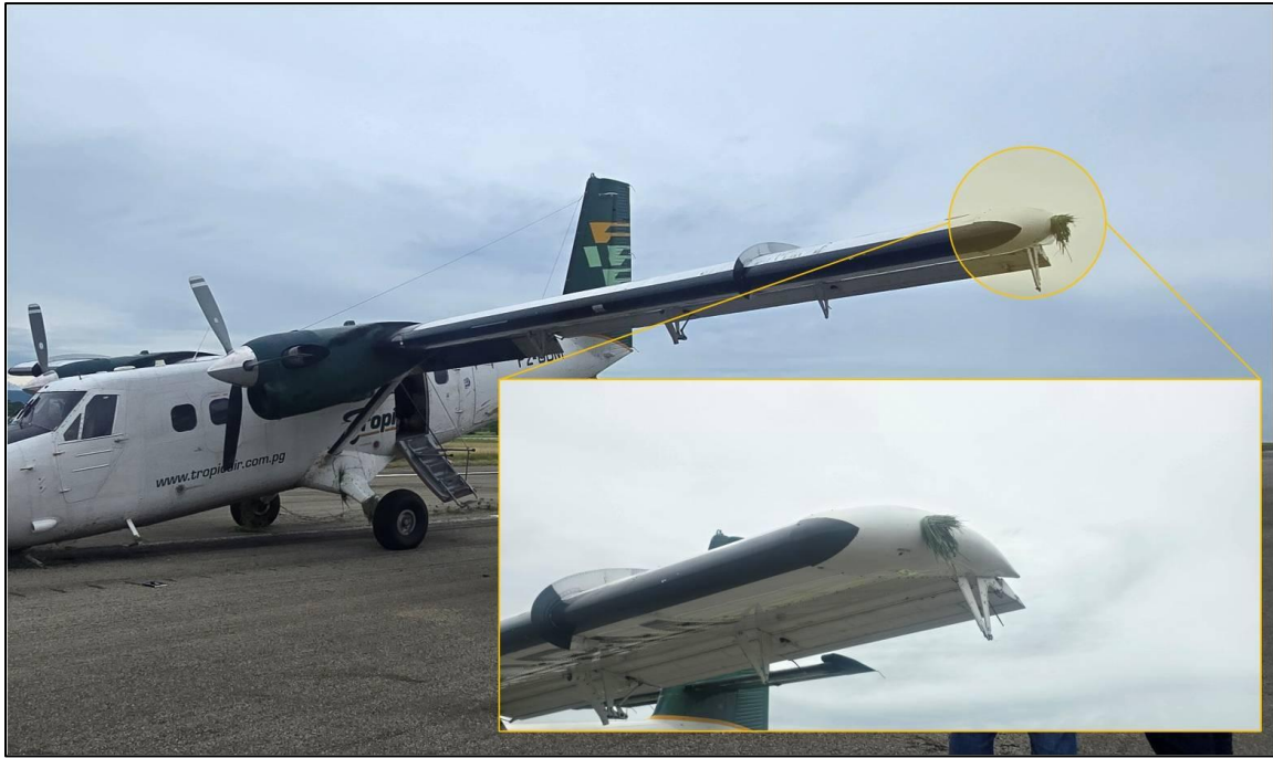
Figure 11. Vegetation (grass) lodged in the left wing-tip of P2-BBM.
