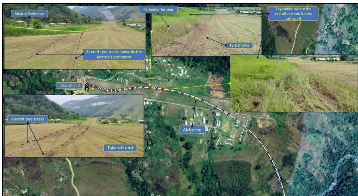
Figure 10. Overview of P2-BBM track along RWY 09 - Tapini Airstrip.
