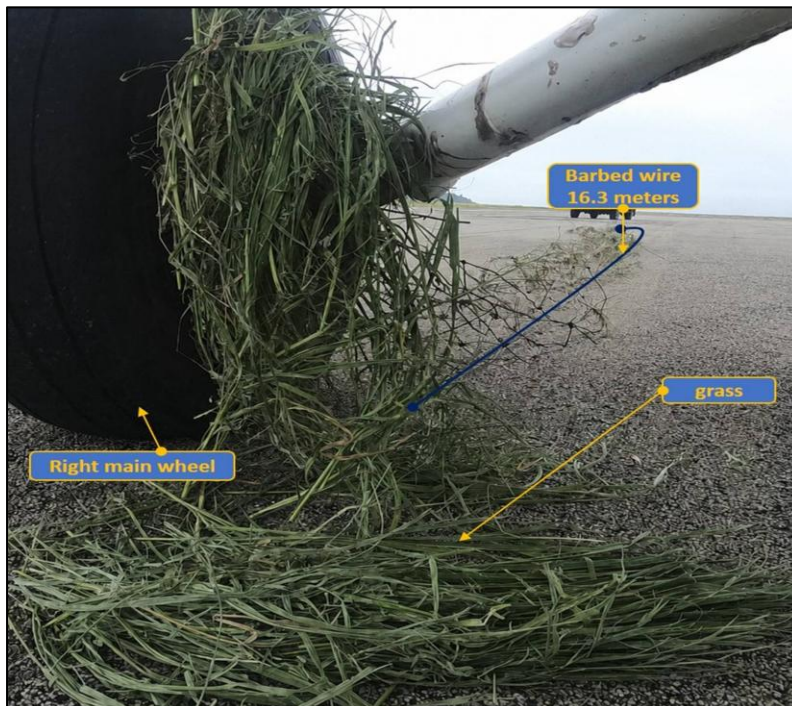
Figure 12. Vegetation (grass) barbed and mesh wire lodged on the Right Main Landing Gear (MLG) of P2-BBM at Jackson International Airport.
